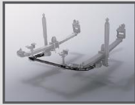
Stabilizer The stabilizer have been lengthened and feature a link bracket, maintaining high effectiveness and stability.
