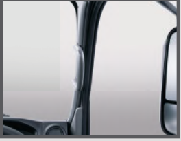
Wide View Pillars The front pillars are designed to be as narrow as possible to ensure a nearly uninterrupted view, allowing the driver to easily see pedestrians and cyclist, without any compromise in structural integrity.
