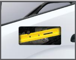
Door Impact Beams The side impact beams built into the doors of 300 Series increase the level of protection for driver and passenger in the event of a collision from the side.
