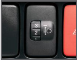
Headlamp Leveling Switch The Headlamp Leveling Switch can be used to adjust the headlamp illumination distance.
