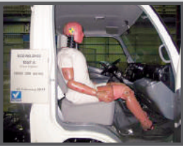
EGIS Cab (Emergency Guard Impact Safety) The EGIS Cab Design is one of HINO'S passive safety features, enhancing the rigidity of the cab.
