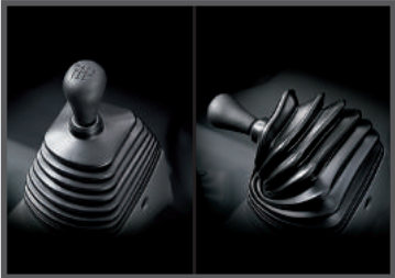
Folding Type Shift Lever The shift lever and side lever fold down, making it easy to move around the driver compartment.
